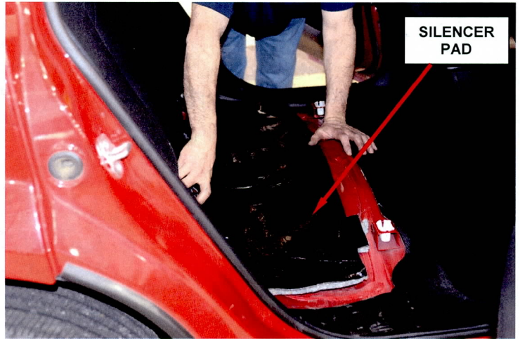
Figure 6 – Install Seat Cushion Silencer Pad
