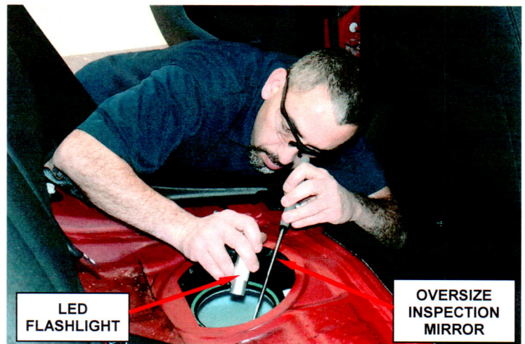
Figure 4 – Inspect Bottom of Control Valve with Oversized Inspection Mirror and LED Flashlight
