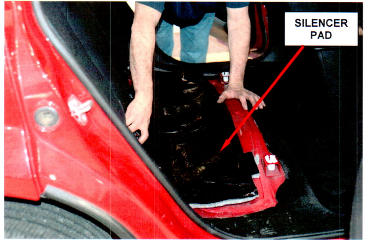
Figure 6 – Install Seat Cushion Silencer Pad
