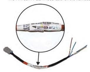
NOTE: Remove the part number label to make sure that if a replacement subharness is ever needed, the wrong part will not be ordered.
