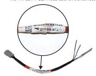
NOTE: Remove the part number label to make sure that if a replacement harness is ever needed, the wrong part will not be ordered.
