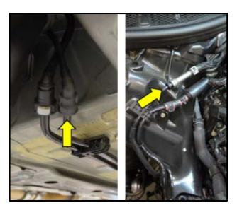
the front and the rear of the fuel supply line <arrows>.
