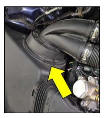
Disengage the intake tube from the air filter housing <arrow>.
