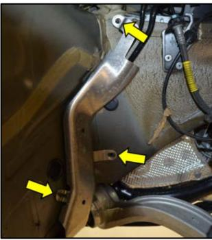
Reinstall the fuel line shield and mounting nuts <arrows>.
