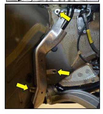
Disconnect the fuel supply line near the right front strut tower <arrow>.
