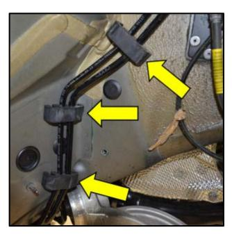
Remove the three rubber insulators from the fuel line assembly <arrows>.
