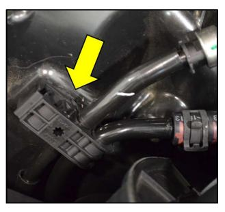
Position and install the mounting clip at the top end of the fuel supply line and evaporative emissions line <arrow>.
