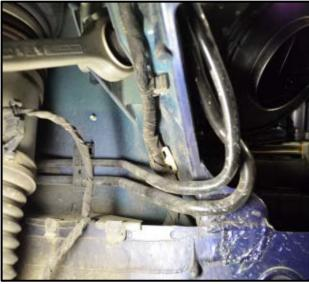
TIP: At this point in the repair process, note the routing of the fuel supply line and evaporative emissions line behind the front strut. Take photos if necessary. When the fuel line is reinstalled it must be routed in exactly the same location and orientation in order to fit properly.
