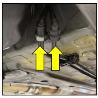
Disconnect the evaporative emissions line and the fuel supply line at the rear quick release connections <arrows>.
