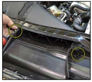
Remove the two mounting screws from the air intake tube <circles>.
