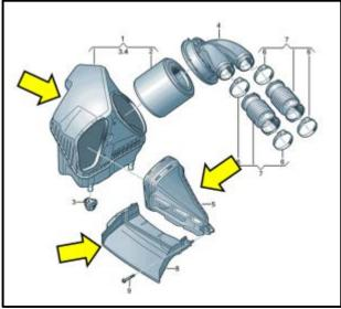
Remove the air filter housing and inlet ducts <arrows>.
