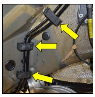
Install the three rubber insulators onto the fuel supply line and the evaporative emissions line <arrows>.
