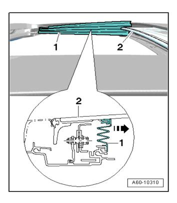
Pull off trim <1> from sunroof panel <2> completely toward vehicle interior and fold it downward and away.
