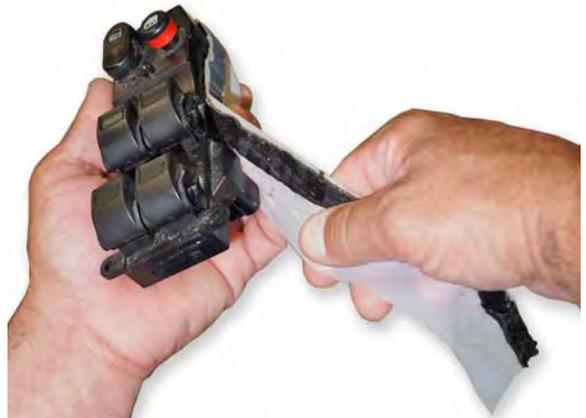
7. Check for corrosion or melting on the switch side and the harness side of the 3P and 20P connectors:
