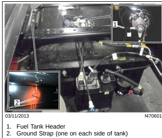
Fig. 1, Fuel Tank Electrical Connections and Hoses
