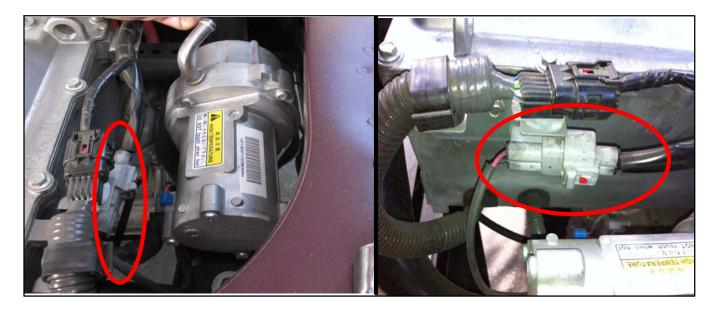
6. Unclip the vacuum pump electrical connector mount from the vehicle's body.
