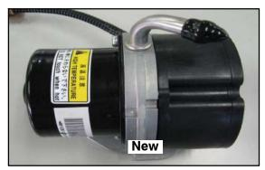
10. Reattach the wire harness clip to the bracket first, and then reinstall the three 10mm bolts. Doing so will ensure the vacuum pump is installed correctly to the bracket.
