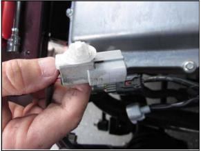
6. Unclip the vacuum pump electrical connector mount from the vehicle's body.
