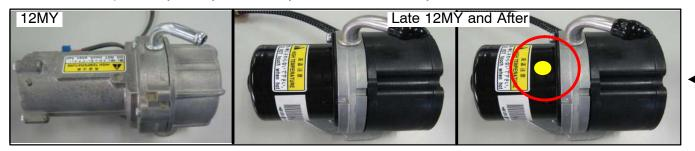
**NOTE:** The replacement vacuum pump has a two-tone exterior (black and silver) with a yellow mark on the body along with a white mark on the top cover near the "Mikuni" insignia as shown below.
