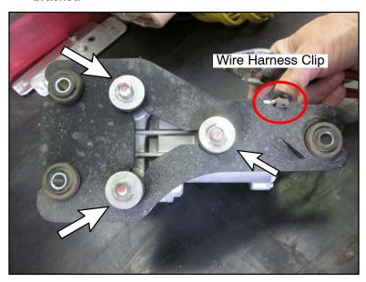
9. Replace the vacuum pump with the new unit.
