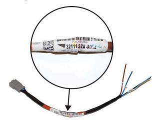
NOTE: Remove the part number label to make sure that if a replacement subharness is ever needed, the wrong part will not be ordered.
