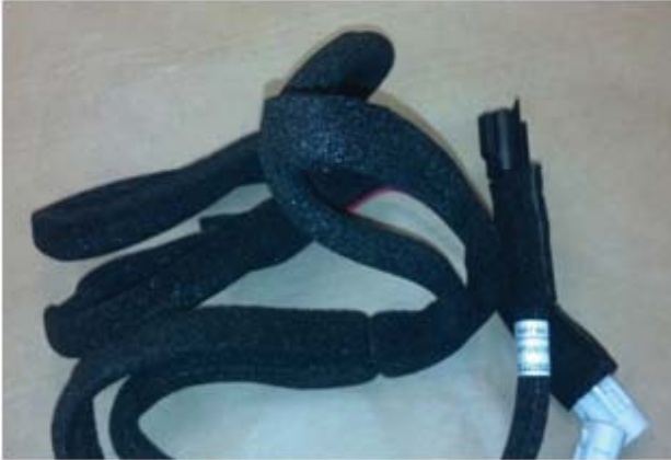
No in-line fuse installed
