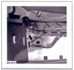
9. A CAUTION: Make sure that the ground cable is fully secured in the area of the luggage compartment lid latch, so that the ground cable cannot come in to contact with the latch.
