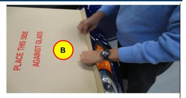
With sunroof shade completely open, place interior template against sunroof glass. Interior template <u>must</u> be placed over sunroof track.
