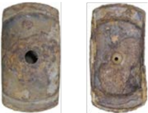
Obvious Rust Corrosion
