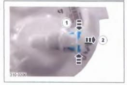
14. A CAUTION: Make sure that the new O-ring seal is installed to the fuel tank fuel outlet mounting flange; failure to follow this instruction may result in damage to the vehicle.
