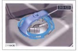
11. A NOTE: Hold the fuel tank fuel outlet mounting flange above the fuel tank aperture and allow any fuel within the fuel tank fuel outlet mounting flange to drain back in to the tank before attempting to withdraw it through the vehicle interior.
