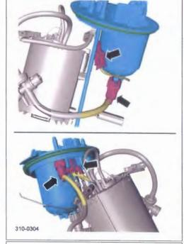
Remove and discard the blanking plug from the new fuel tank fuel outlet mounting flange.
