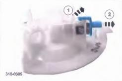
Remove and discard the clip from the new fuel tank fuel outlet mounting flange.
