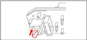
c) Push the window lock button so that it is in the down position.
