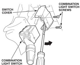
Using a flat-tip screwdriver wrapped with electrical tape, slightly lift the switch cover, then remove the switch, and discard it.
