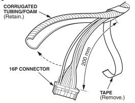
8. Locate the RED/WHT wire in the 16P connector. Then measure 150 mm from the end of the connector, and cut the RED/WHT wire there.
