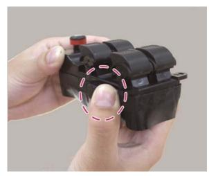
Pinch the butyl tape at the connector so that it sticks properly, with no creases in the butyl tape. Make sure the holes by the connector are covered.
