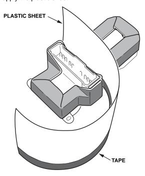
10. Wrap the plastic sheet around the connector, peeling off the backing paper.
