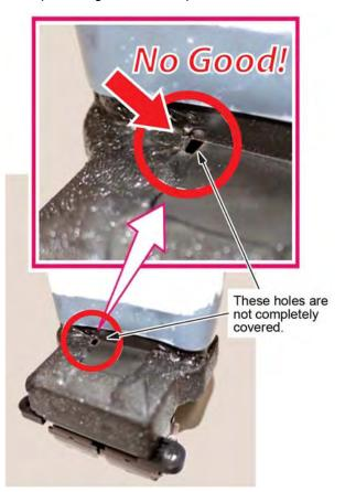
12. Reinstall the driver's switch panel into the door panel. Make sure the plastic sheet is not crushed, crumpled, or folded when you reinstall the switch panel in the door.
