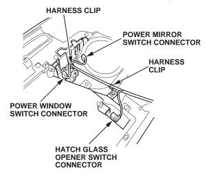
Push up on the bottom of the power window switch to release the clip and the hooks, then remove the switch.
