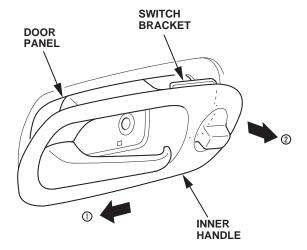
4. Disconnect the power door lock switch connector. Disconnect the inner handle rod, and remove the inner handle.
