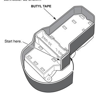
3. Wrap the tape counterclockwise around the entire switch, peeling off the backing sheet as you go.
