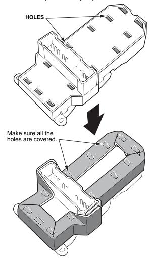
9. Align the tape on the plastic sheet to the starting point of the base of the connector as shown, then apply the plastic sheet.
