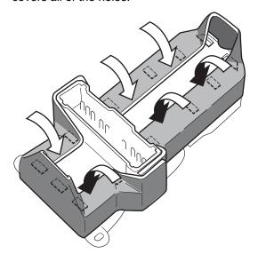
7. Fold the butyl tape at the top and bottom areas of the switch and stick it to the rear face. Make sure the holes are covered.
