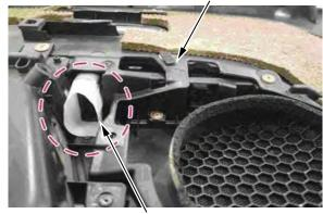
Be sure the plastic sheet on the window switch is not crumpled.
