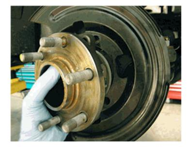
7. Reinstall the splash guard while aligning the wheel speed sensor opening in the splash guard to the steering knuckle.
