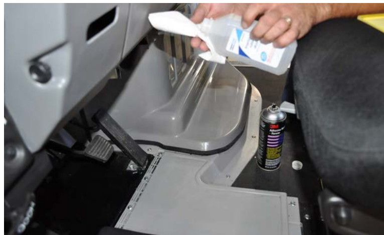
Clean floor and mat with alcohol
