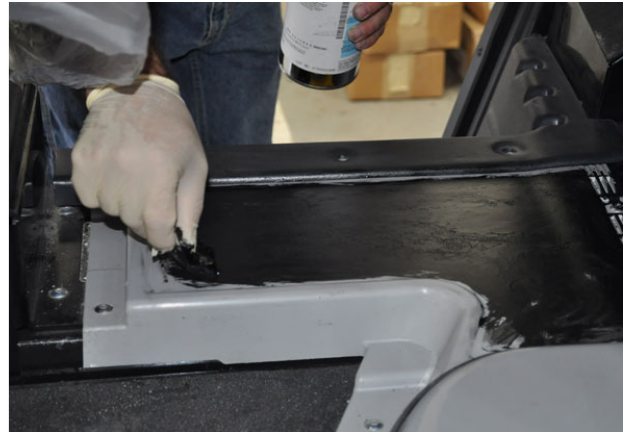
Primer application to mat and floor panel
