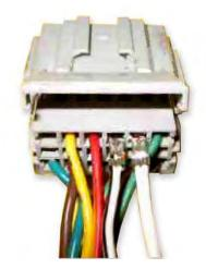
5. Wrap the connector with foam tape (EPT sealer 3T), and reinstall the harness.
