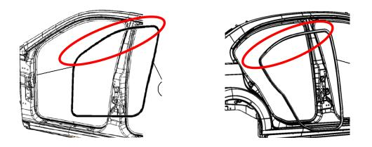
5. Gently pull down on the headliner between the vehicle pillars at the front door and at the rear door to expose the side curtain airbag.
