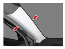
3. Remove grab handle by pulling down to expose mountings. Release screw covers and remove (x2) screws securing grab handle to body. Refer to Service Manual Sections 82 and 84 (FTR 82204002).
