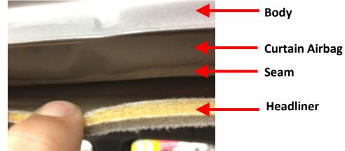
9. Obtain a clear view of the side curtain airbag and confirm proper installation along the entire length of the curtain airbag.
