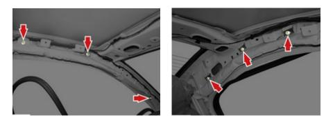
16. Once installed correctly, torque securing bolts to 9 Nm (7 lb/ft) and reassembly other components in reverse order of removal.
