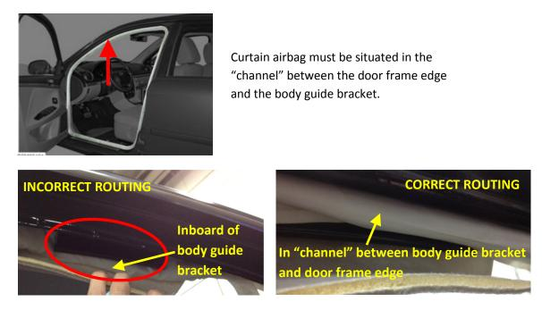
If found to be installed inboard of the bracket, photograph the area and contact CODA TAC prior to continuing with repair. CODA TAC can be reached at 888-718-5046.
