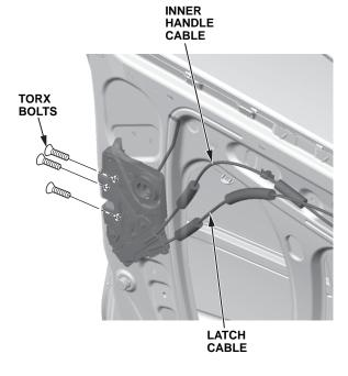
• Lower the door latch to slide it off the outer handle rod, and remove it.
