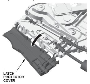
Disconnect the inner handle cable and the latch cable from the front door latch.
