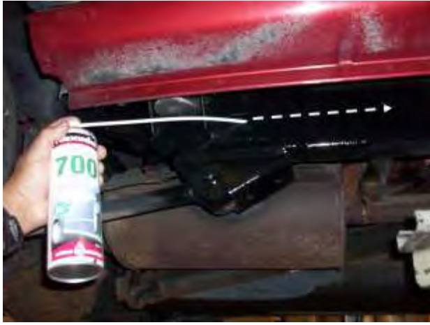
Figure 10 – Frame Hole Toward Front (300 mm)
