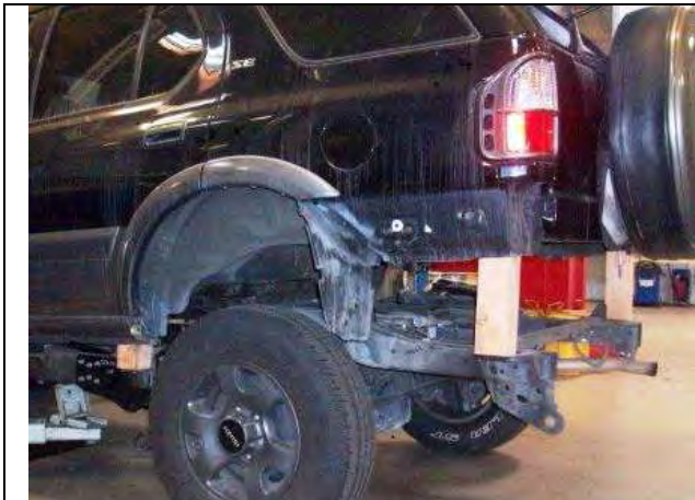
Figure 45 – Wood Blocks Installed at #5 Body Mount
