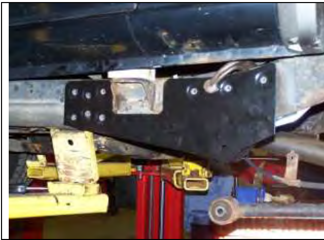
Figure 51 – Type “B” Bracket (temporary installation)
