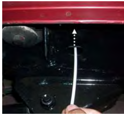
Figure 13 – Frame Hole Up
