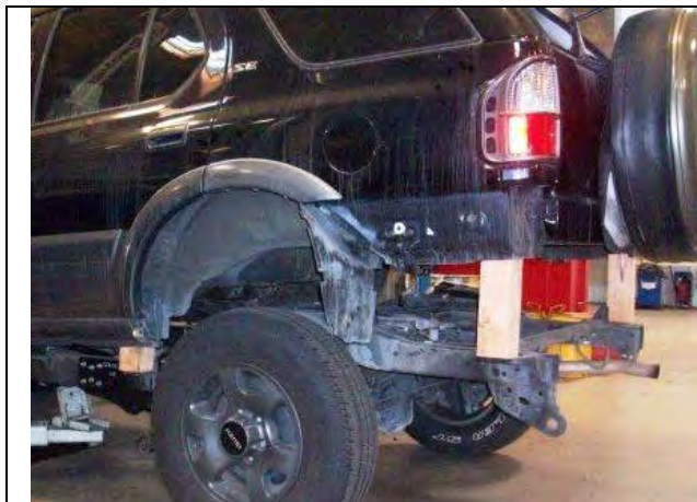
Figure 45 – Wood Blocks Installed at #5 Body Mount
