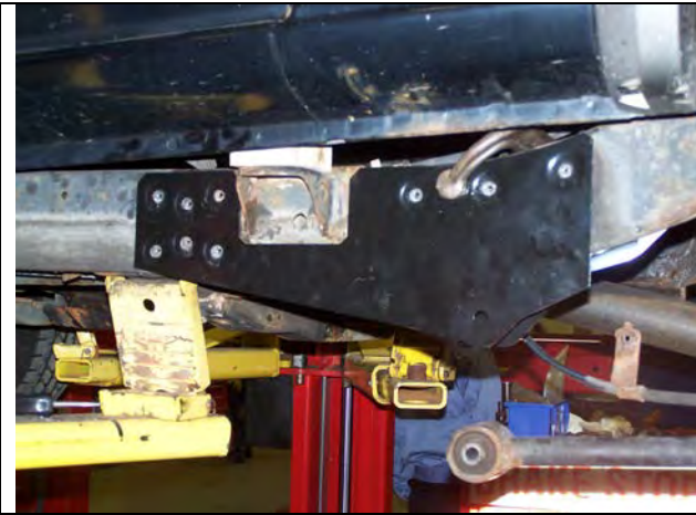
Figure 51 – Type “B” Bracket (temporary installation)
