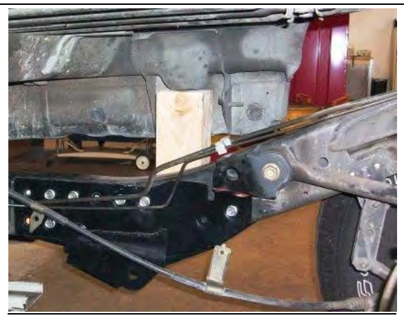
Figure 46 – Wood Block Installed at #3 Body Mount
