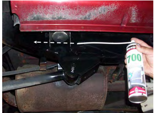
Figure 11 – Frame Hole Toward Rear (300 mm)
