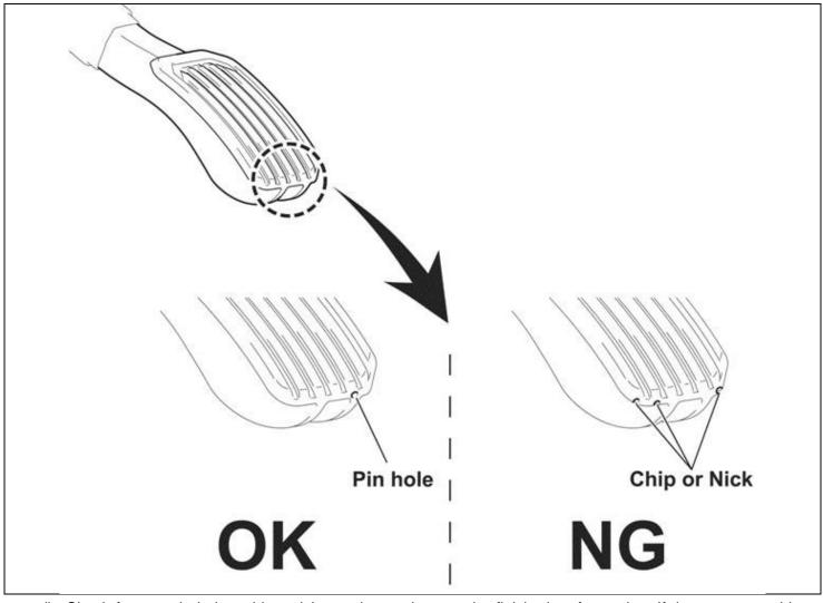
d) Check for any pin holes, chips, nicks or sharp edges on the finished surface edge. If there are any chips, nicks or sharp edges, file them to make them smooth.
