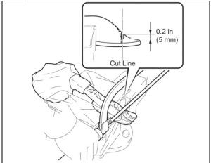
b) Using a hack-saw, cut the pedal 0.2 in (5 mm) to create a guide cut for the reciprocating-saw.
