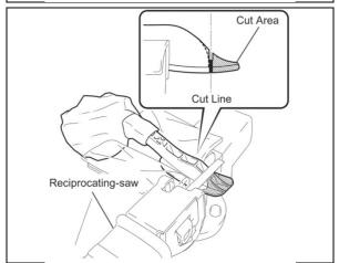
c) Using the reciprocating-saw, cut off the lower section of the pedal as illustrated.
