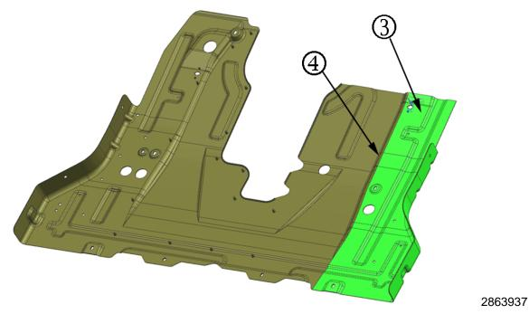
9.3 Using a Sawzall or equivalent, cut the left side of the engine shield (3). Cut the engine shield along the feature line (4) from front to rear. Refer to illustration.
