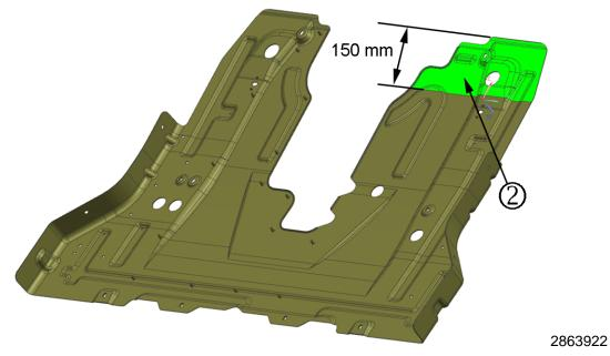
9.2 Using a Sawzall or equivalent, remove 150mm (5.9 in) from the left side of the engine shield. Refer to the light green portion (2) of the engine shield in the illustration.
