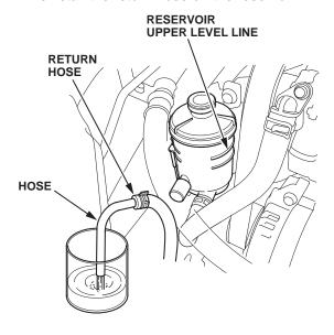
2. Remove the P/S pump outlet hose from the P/S pump, then plug the outlet hose and the P/S pump. Remove the P/S feed hose from the clamp.
