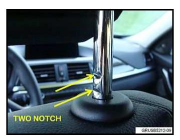
5. Before proceeding ensure the headrest is still in the two notch position as shown, and then proceed to the next step.
