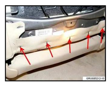
4. If the reusable push pins were removed, you must remove the seatback leather from the retaining tabs to recover the two center pins. Bend the seat tangs downward and pull the leather off in an upward/rearward direction. Collect the two reusable pins and install the leather to the tangs through the original holes; and then bend the tabs upward to secure.
