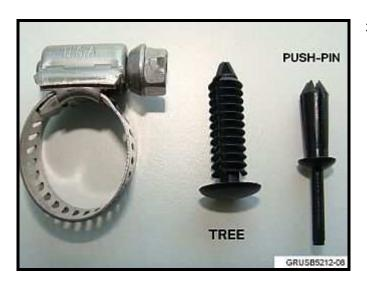
3. For the rear panel, two types of retaining pins were used. For cars produced prior to mid-February 2012, the "tree"type pins were used, and must be replaced. Carefully remove this type, and discard. From mid-February 2012 forward, the newer expanding rivet "push pin" type have been used, and are reusable. Push in the center pin through the clip until it falls out, and then carefully remove the retainer.
