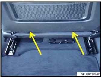
Position the seat to the uppermost height setting and the forwardmost seating and backrest position to locate the two retaining pins. Remove the rear panel on the front seat backrest. Refer to Repair Instructions "52 13 198 Remove and refit/replace the rear panel on the left or right front seat backrest."
