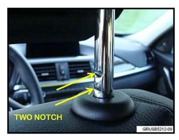
Raise both front headrests to the maximum height position, and inspect the chrome post. If only two notches are visible, no further action is required. If more than two notches are visible, position the headrest so that only two notches are showing, and then proceed to the next step.
