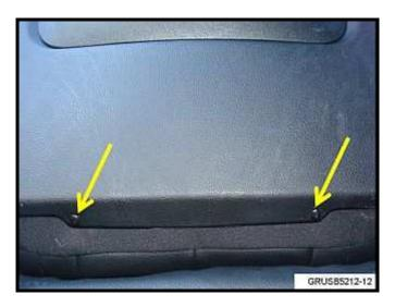
7. Refit the rear panel and secure with two retaining pins. If the original pin was a "tree" type, install a new "tree" type. A "push pin" type can be reused by inserting the retainer to the seat panel and seat frame; then insert the center pin back into the retainer, until flush.
