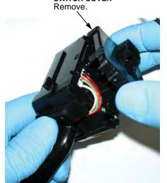
19. As shown below, route the wire tie from the kit through the hole in the lower corner of the switch cover. Then use the wire tie to secure the RED/WHT wire (in the section you taped in step 11) to the switch cover. Cut off the excess wire tie.
