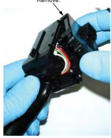
22. As shown below, route the wire tie from the kit through the hole in the lower corner of the switch cover. Then use the wire tie to secure the RED/WHT wire (in the section you taped in step 13) to the switch cover. Reinstall the cover, and cut off the excess wire tie.
