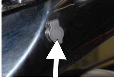
CHARGE AUX BATTERY (DIN)
