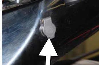
CHARGE AUX BATTERY (DIN)
