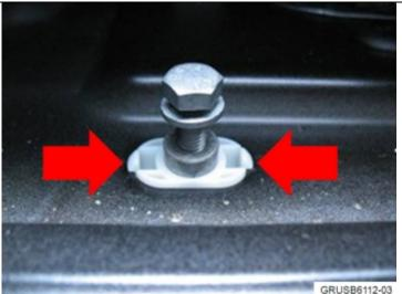
7. Screw the previously removed securing bolt into the lug and pull up, so that both retainers on the clip are locked into the sheet metal.
