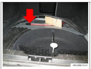
4. **E60, E63, and E64 only:** Prop up the trunk floor trim panel in order to gain access to the battery cable. For the E61, proceed to the next step.
