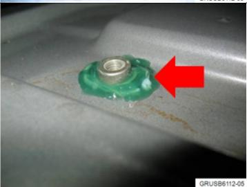
**8.** Coat the area around the lug covering the retaining clip with contact protection grease.
