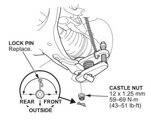
4. Disconnect the lower arm from the knuckle. For more information about removing the ball joint, refer to the service manual, or online using the keywords **Ball Removal**.
