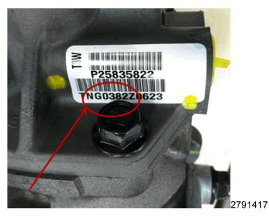
Digits 4-8 of the TNG number signify day and year of the build. The digits in the 4-8 position in the illustration are 0382, which means the steering gear was built on the 38<sup>th</sup> day in 2012. This steering gear would require replacement of the steering gear pitman shaft and housing.
