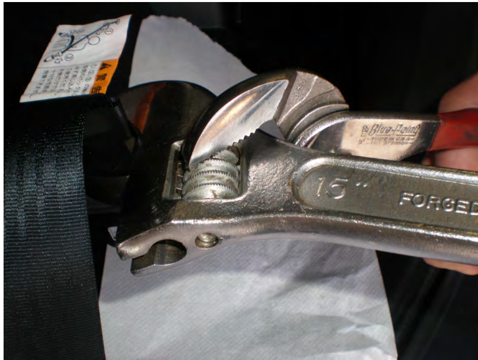
Figure 9: Seating the Tack Collar
