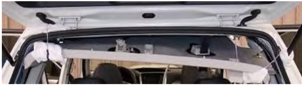
Headliner supports in place
