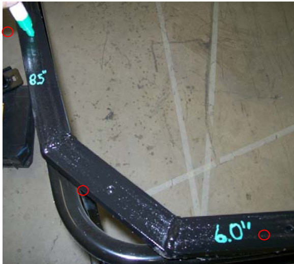
Figure 6: Seat frame reinforcement bracket –seat frame side view The longer bracket side fits on the back of the seat (as shown)
