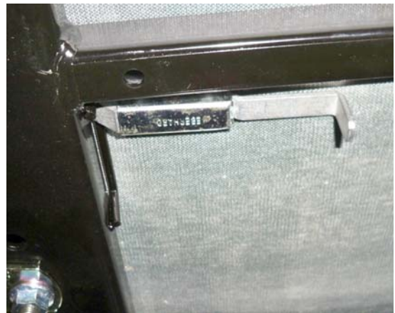
Figure 4: Self latching device – seat underneath view
