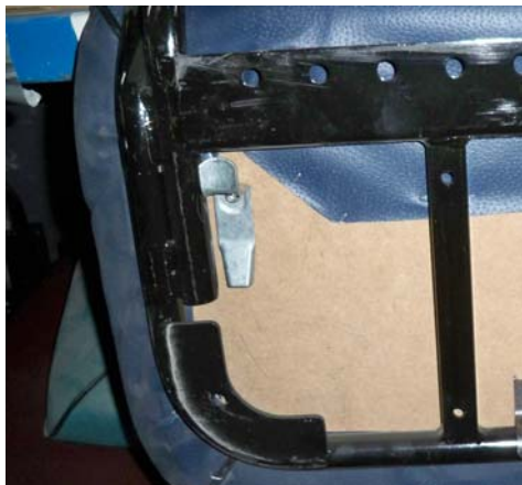
Figure 3: Quarter turn bracket – seat underneath view
