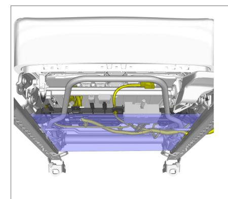
Note! Extra cable length must be secured using cable ties.
