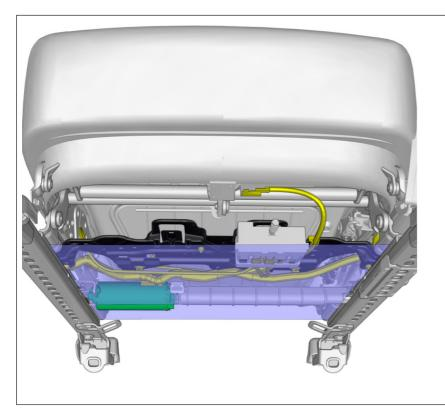
Note! Extra cable length must be secured using cable ties.
