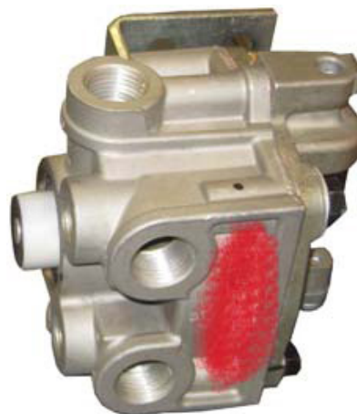
Figure 5: Bendix removed ATR-6 valve
