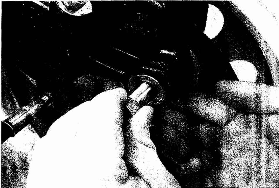
Photo 11 - To Align the Caliper Correctly with the Threaded Hole In the Mounting Bracket Lift the Caliper Slightly. You Will Feel The End of the Pin Align With That Threaded Hole.
