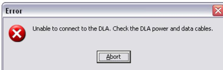
You must connect the Bus/ DLA to the computer before running FlashLoader.exe, or make sure the DLA/ Cluster has been installed first (or reconfiguring for a new USB port)
