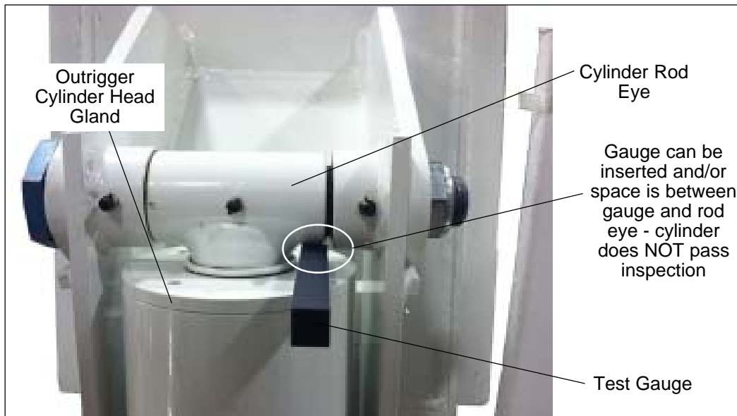
Figure 2 — Using The Test Gauge On The Outrigger Cylinder
