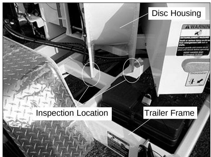
Figure 2 — Close-up Of Inspection Locations
