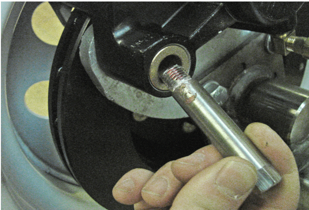
Photo 20 - Re-Install the Slider Pin Into The Caliper.
