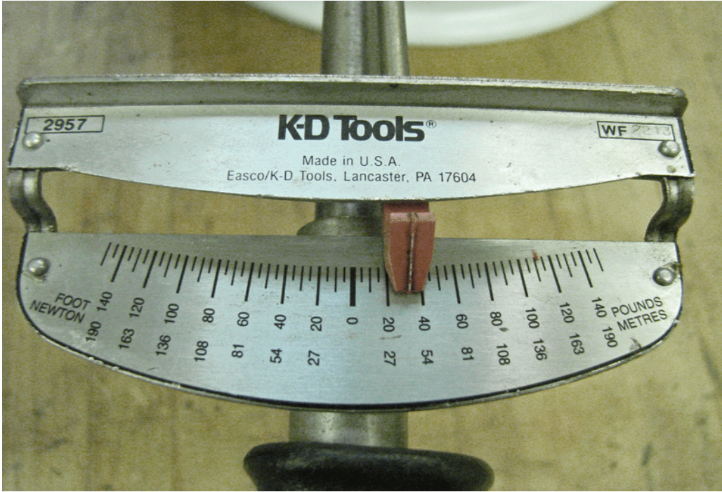
Photo 14 - Torque the Slider Pin to 35 Ft. Lbs. You Are Now Finished Re-Installing the First Slider Pin.
