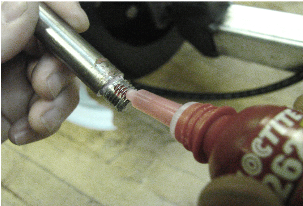
Photo 17 - Apply the Liquid Loctite 262 to the Threads of the Slider Pin As Shown.
