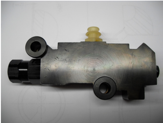
Fig 7: Wilwood Proportioning Valve Part #260-11322
