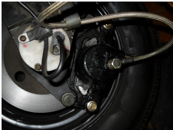
Fig. 5: Braided Stainless Steel Brake Line
