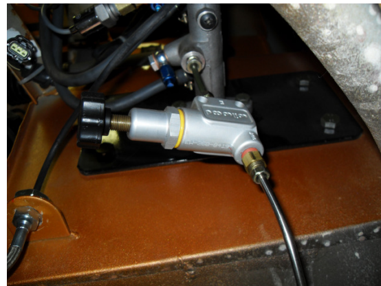
Fig. 6: Wilwood Proportioning Valve Part # 260-8419
