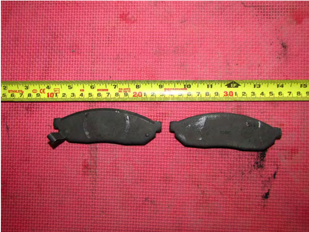
FIGURE 23. RIGHT REAR BRAKE PADS
