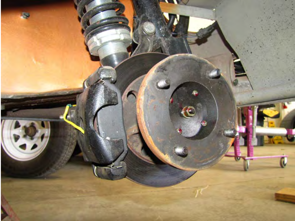
FIGURE 15. FRONT BRAKE WITH THERMOCOUPLE INSTALLED
