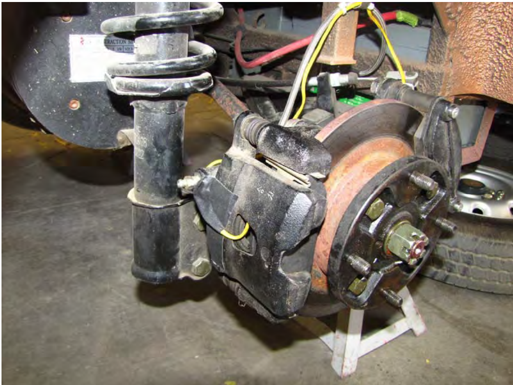
FIGURE 20. RIGHT REAR BRAKE WITH THERMOCOUPLE INSTALLED
