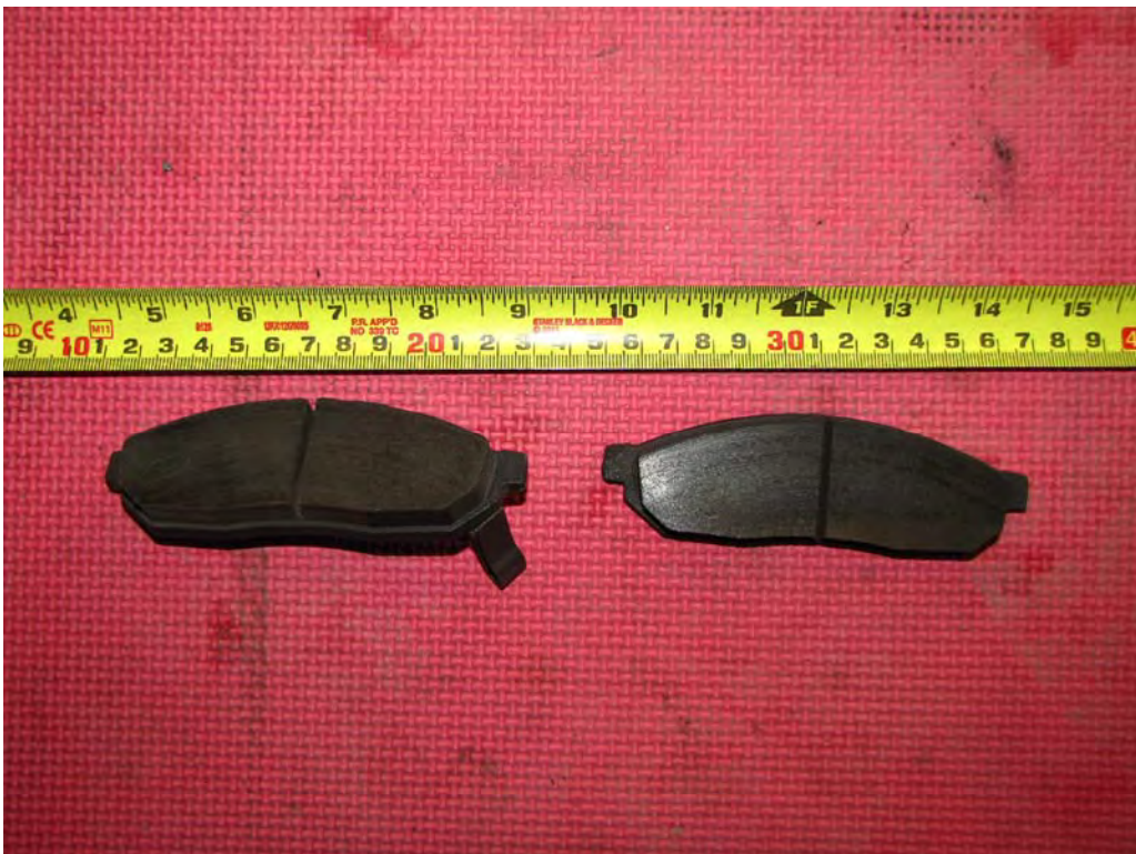
FIGURE 22. RIGHT REAR BRAKE PADS
