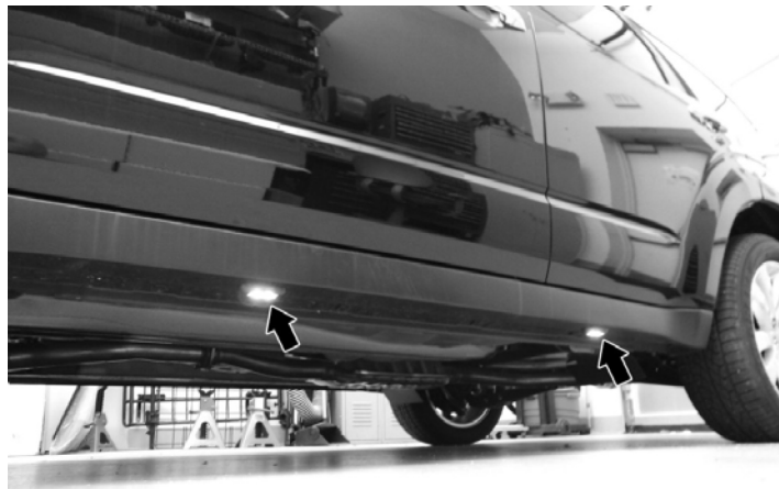
CHECK FOR FUNCTIONING PUDDLE LIGHTS
