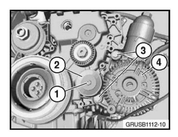
3. Remove cover (1) from Deflection pulley (2) to access the mounting bolt. Remove the deflection pulley (2).
